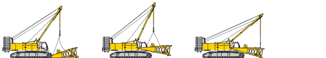
Unloading and assembly of boom foot
